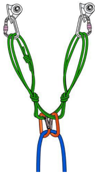
Example: Quad Anchor - Self-Adjusting Multipoint Anchor w/ force limiting knots
